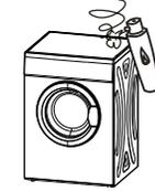
Do not wash or dry articles that have been cleaned in, washed in, soaked in or spotted with combustible or explosive substances ( such as wax, oil, paint, gasoline, degreasers, dry-cleaning solvents, kerosene, etc.).
